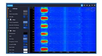
Spectrogram / Waterfall view for the identification of frequency hops, measuring of pulse rate, analysis of time-variant spectra and the tuning of a VCO
